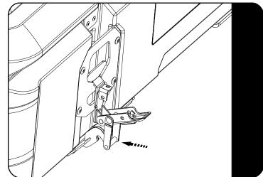
Place the Latch Loop over the Catch Hook on the Base Plate.
