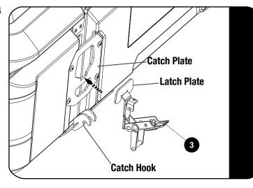
Before attaching the Case to a roof rack, inspect the Latch Plates for damage or insecure fit.
