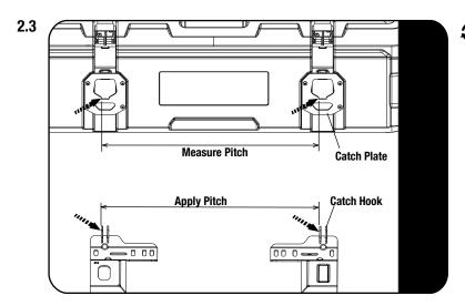
Measure the pitch on the Pelican Case Catch Plates as shown.
