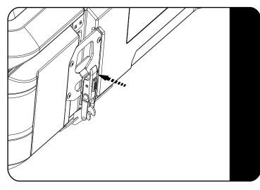
Close the Latch to secure the Pelican Case onto the rack.
