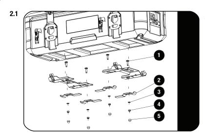
Loosely fit two Tubular Rack Clamps (Item 2) underneath each Pelican Case Base Plate using four M8 x 30 Carriage Bolts, four M8 Flat Washers and four M8 Nyloc Nuts (Item 1, 3, 4).
